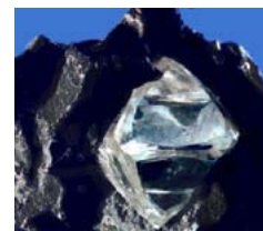
Diamond is the hardest natural material, and has a Mohs hardness of 10.
